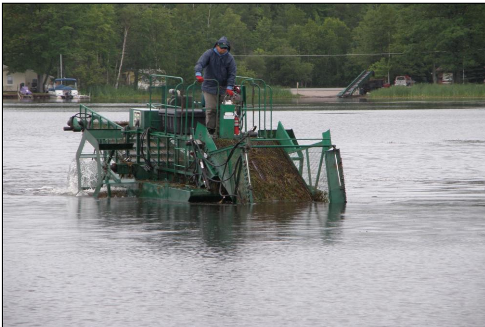
Figure 43. A mechanical harvester used to remove aquatic plants.
