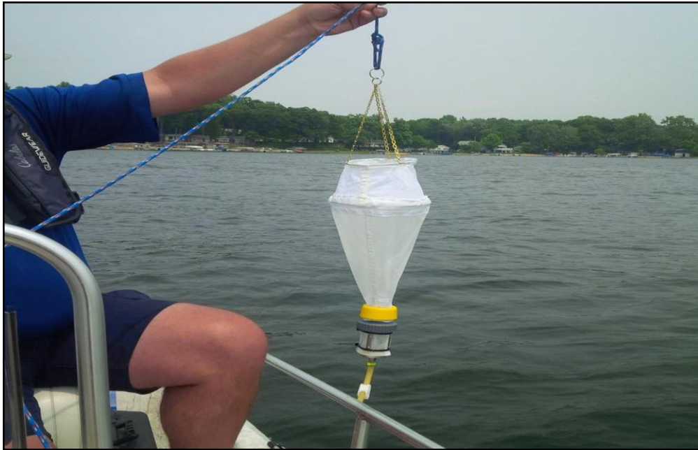
Figure 34. A zooplankton collection tow net.
